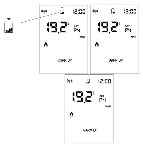
The arrows will light up in sequence to signal the need for pellet loading.
