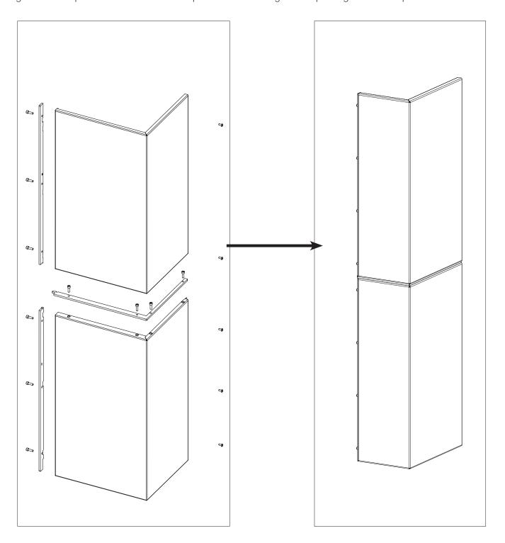
Insert the assembled right-hand side panel.
