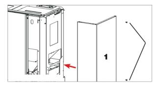
Fasten it to the top and right-hand sides with a screw.
