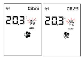
You can confirm the setting with the button and then move to the next fan, if present, otherwise you can exit the fan setting page and "SET" will stop flashing. Alternatively, wait 5" without pressing any button to exit the fan setting, and "SET" will stop flashing, even if there are other fans.
