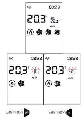
You can confirm the setting with the button and then move to the next fan, if present (only for PLUS ducted versions), otherwise you can exit the fan setting page and "SET" will stop flashing.
