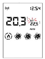
After setting the installation room temperature (or with the room power in manual mode), wait 5" without pressing any button and "SET" will flash then you will exit the settings page.
