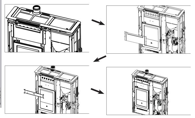
Position the four metal side elements (7, 8, 9, 10) from the bottom. Each element snaps into place and then bolts on
